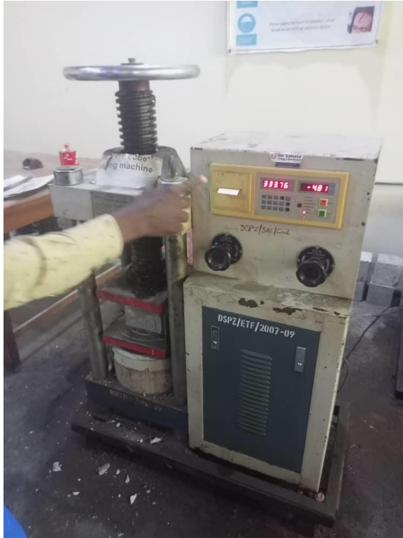
Figure 1. The crushing of the concrete cube.
