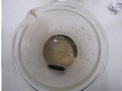
Figure 3. The slurry stayed at lowest part following one day of mixing.
