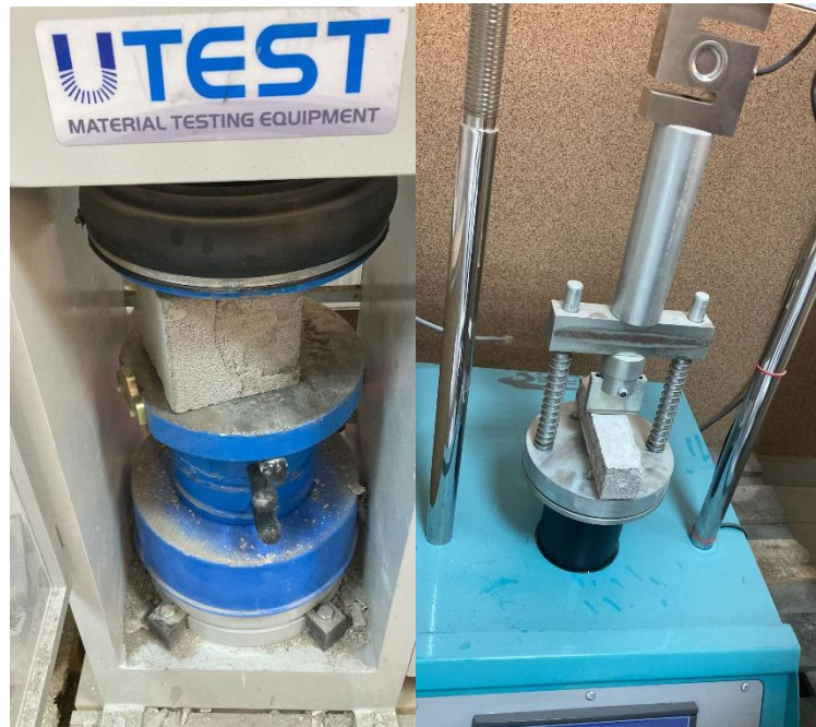
Figure 2. Compression and flexural test
