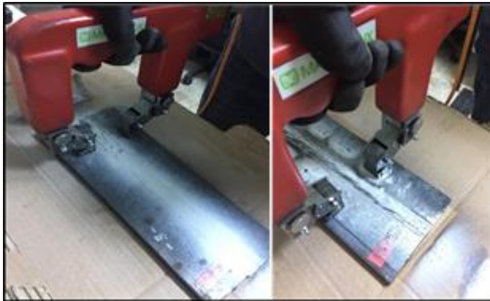
Figure 4. Magnetic particle test application image
