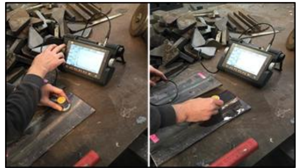
Figure 6. Ultrasonic inspection application image
