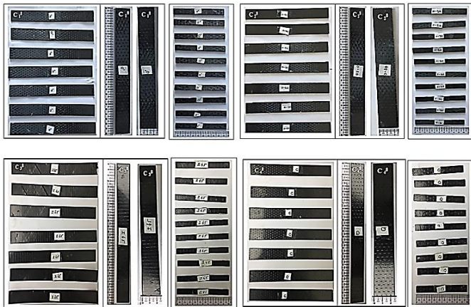
Fig. 3. CFRP composite tensile and three-point bending test specimens with different orientation angles of C_1^8 , C_2^8 , C_3^8 and C_4^8
