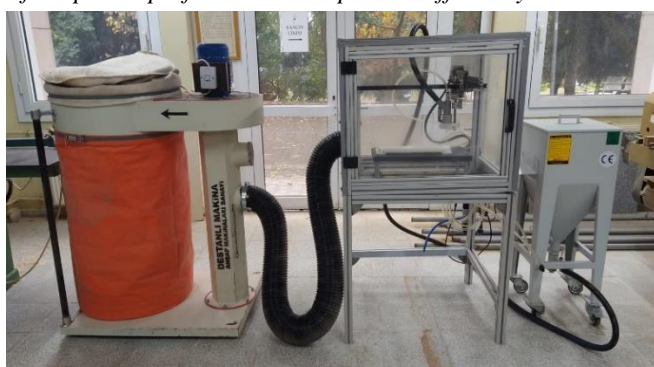
Figure. Representation of the device designed for removing aged layers on wooden surfaces.
