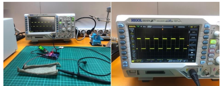
Figure 4. Signal measurement of knitted fabric sample
