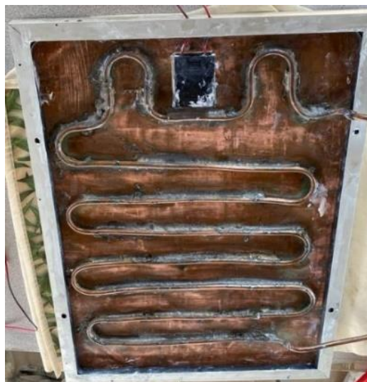
Figure 3. Application of copper pipe on a copper plate and PV panel
