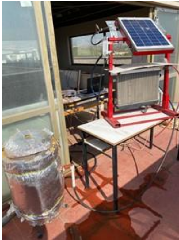
Figure 5. A fan-cooled heat exchanger with PV/T system
