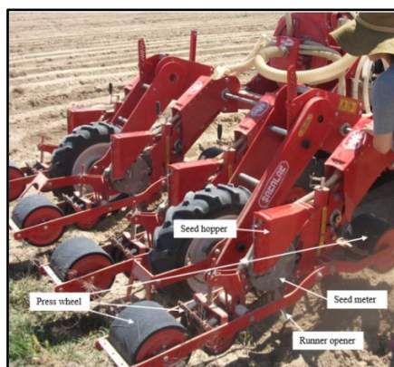
Figure 1. View of pneumatic precision vegetable seeder
