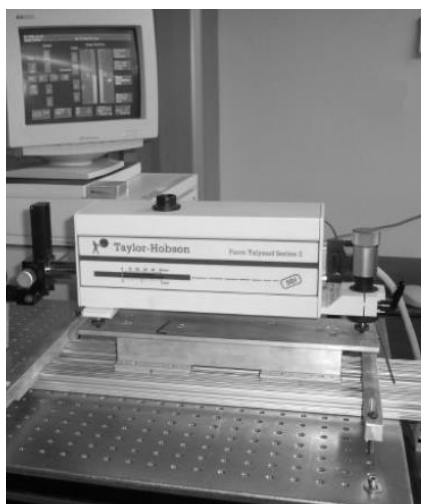
Figure 1. Stylus Profilometer to Quantify Surface Topography
