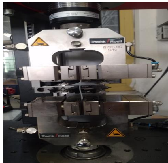
Figure 7. The elongation at break test with a Zwick/Roell Z010 10kN ProLine 739384.
