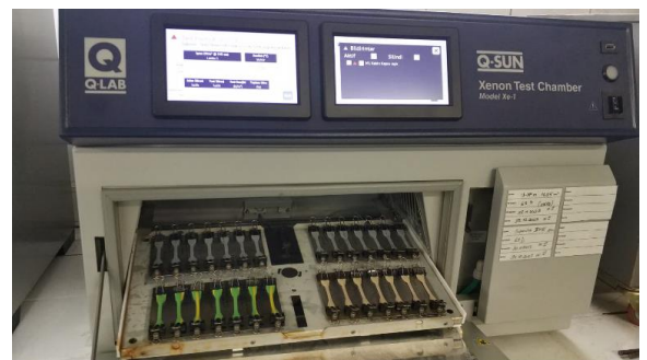
Figure 5. The thermoplastic polyolefin dumb-bell test pieces placement in the Q-SUN Xenon light test chamber.
