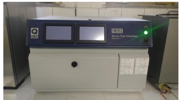
Figure 4. The Q-SUN Xenon light test chamber used for the UV aging test.
