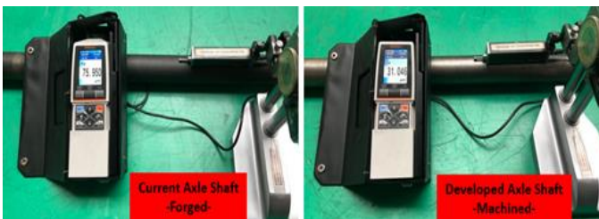
Fig. 6. Comparison of axle shaft surface condition
