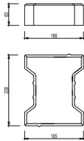
Fig. 2. The dimensions of Interlocking Paving Stones (Iston, 2021).
