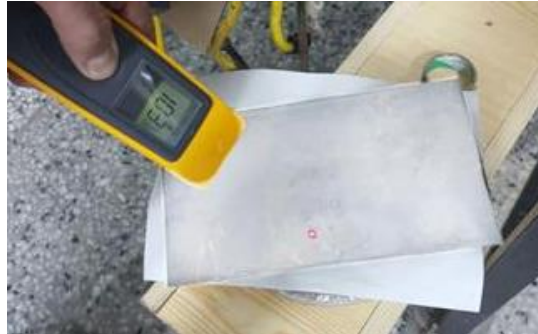
Figure 17. Measuring the temperature of the workpiece over time
