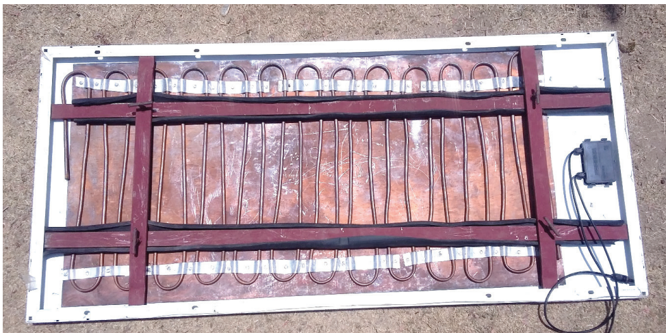
Figure 3. Absorber plate attached with PV module.
