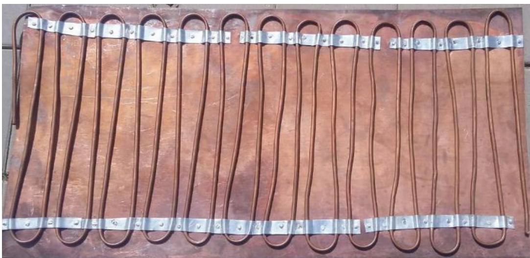
Figure 2. Absorber plate (Copper).
