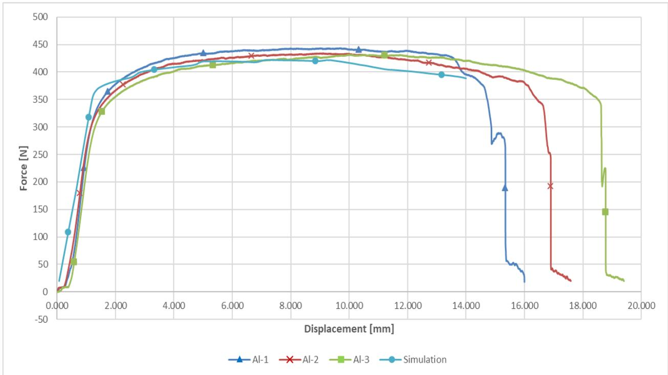
Figure 11. Force displacement behavior obtained from three-point experiment and used in the FEM (ANSYS) simulations.
