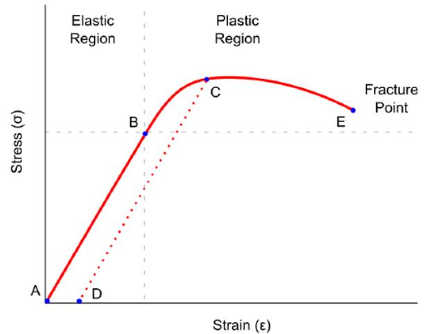
Figure 6. Stress/Strain Graph [16].
