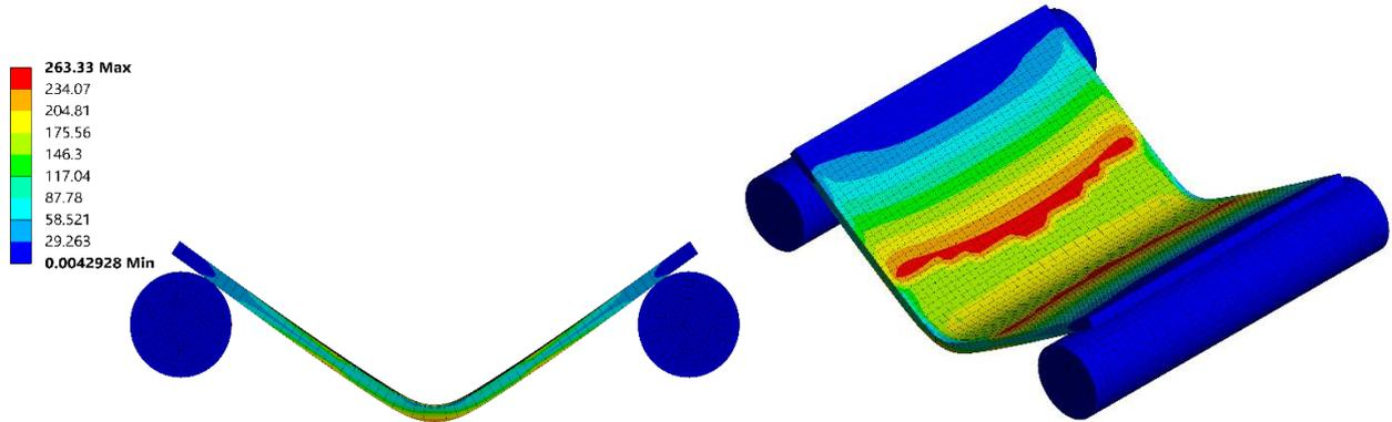
Figure 9. Von Mises equivalent stresses generated in the simulation of the three-point bending test.
