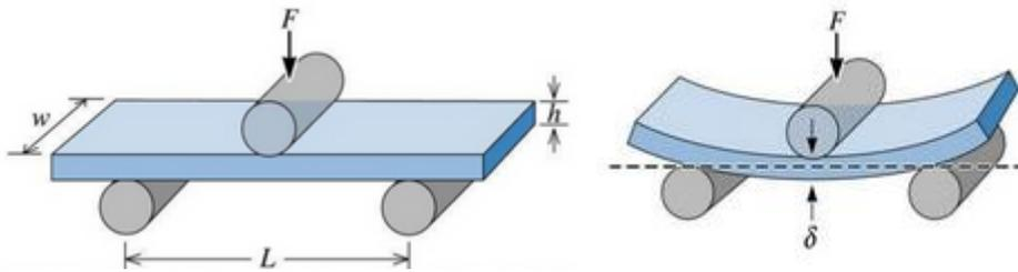
Figure 1. Three-point bending assembly [4].
