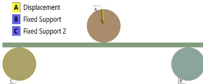
Figure 5. Force direction and contact surfaces
