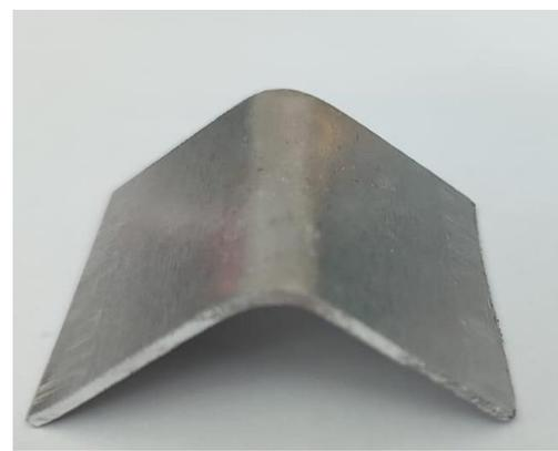
Figure 7. A photograph of the workpiece after the three-point bending test.
