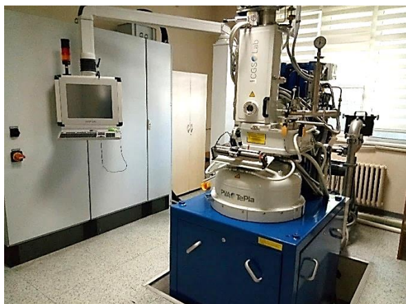
Figure 1. PVA Tepla Czochralski laboratory scale single crystal ingot growth device [13].
