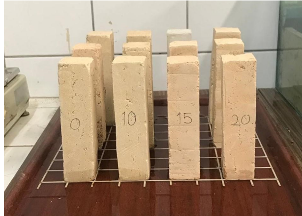
Figure 8. Sprinkler test results: Starting on the left are shown the samples with 0, 0.10, 0.15, and 0.2 ratios of gypsum added in the front row; the same ratios are shown in the middle row but with 0.05-0.10 lime added, with the rear row showing the 0.00 and 0.10 gypsum adobe with 0.025-0.05 lime.
