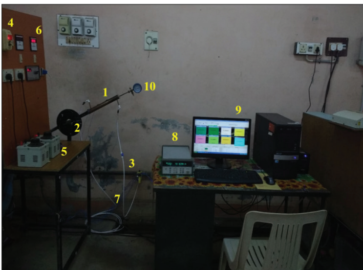
(1: Heat pipe, 2: Inclination arrangement, 3: Water line, 4: Main power supply, 5: Voltage regulators, 6: Watt meters, 7: T – type thermocouples, 8: Agilent data logger, 9: Desktop computer, and 10: Vacuum pressure gauge)
