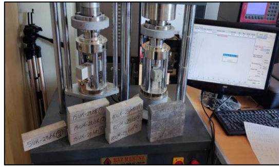
Figure 2. Flexural and compressive strength test
