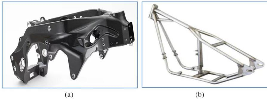
**Figure 35.** (a) Monoblock and (b) Tubular Motorcycle Chassis
