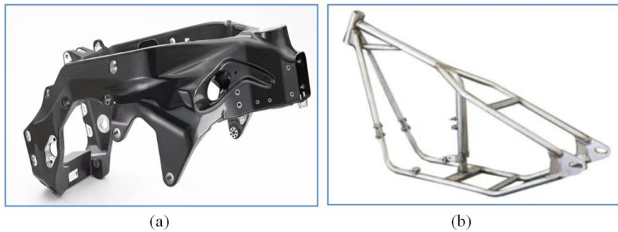
Figure 35. (a) Monoblock and (b) Tubular Motorcycle Chassis
