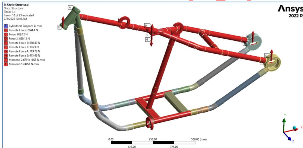
Figure 28. Boundary conditions for frame dynamic load analysis in cornering for Hybrid Frame
