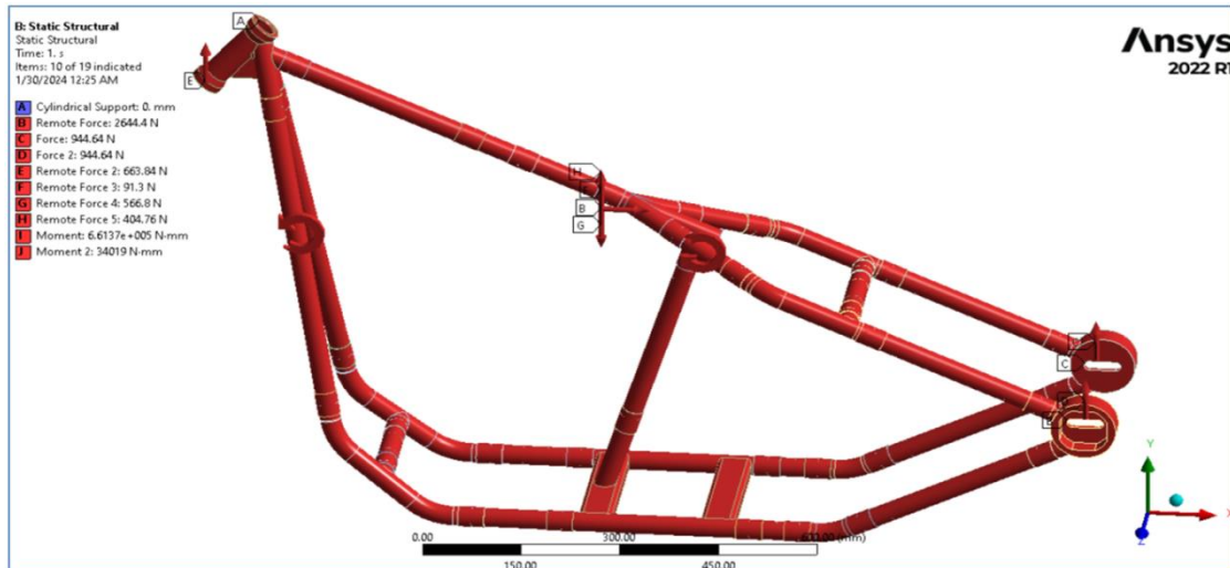
Figure 18. Application of boundary conditions in acceleration for Hybrid Frame
