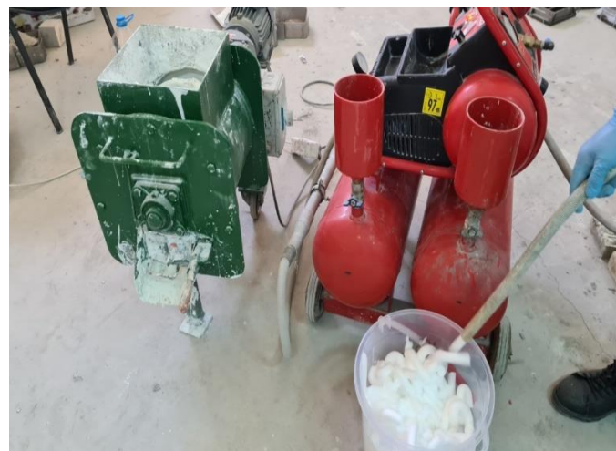
Figure 1. Foam production in a foam generator
