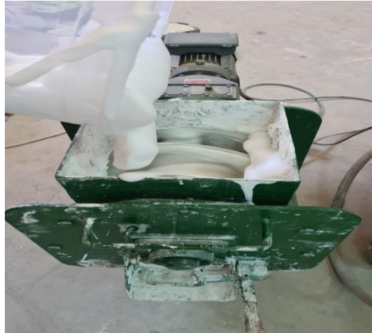
Figure 2. Adding the produced foam to the mixture in a helical type mixer
