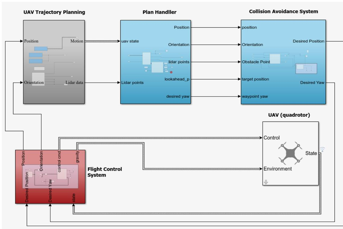
Figure 6. Block diagram of the system simulated in MATLAB Simulink
