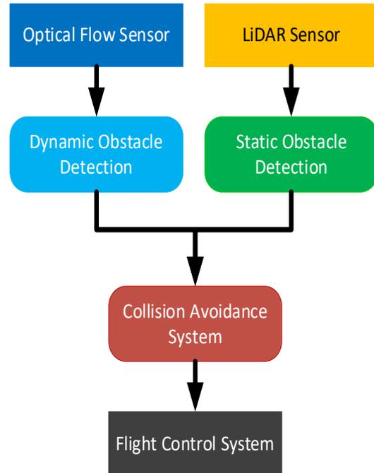
**Figure 2.** The block diagram of Collision Avoidance System
