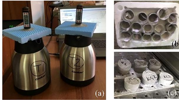
**Figure 2.** Views of the calorimeters (a) that were used in the experiments and test samples (b, c) for the specific heat value
