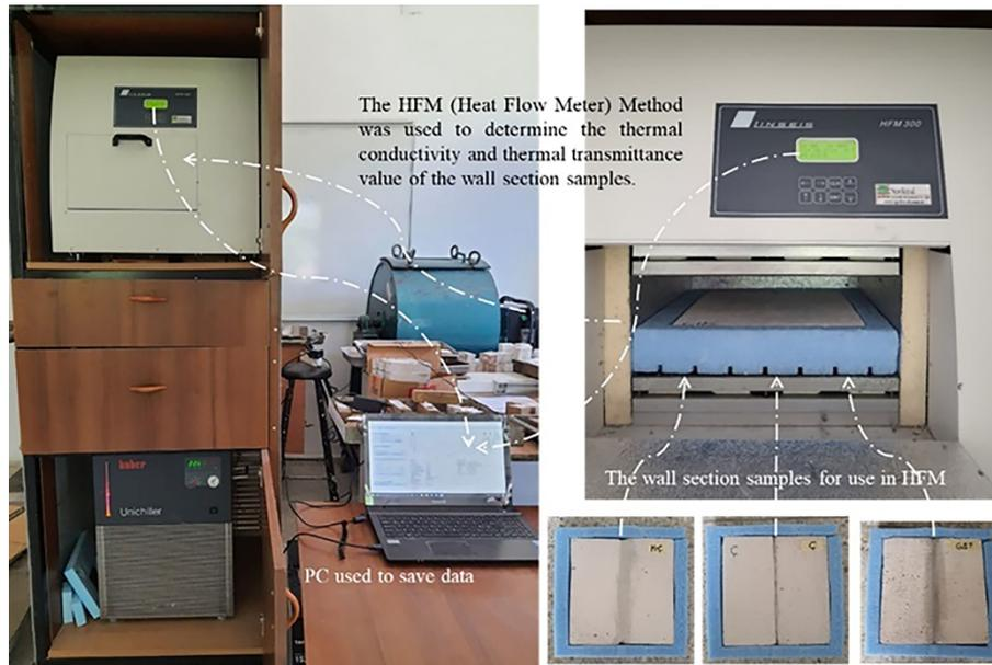
**Figure 1.** Heat flow meter method (coded HFM 300)
