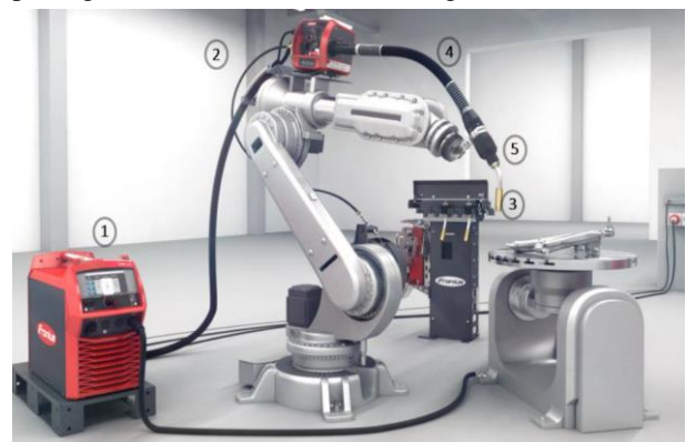
Figure 2. WAAM process components [8]
