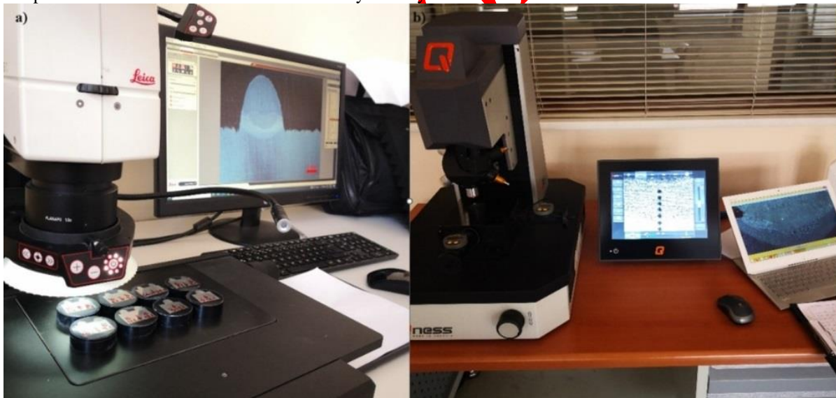
Figure 9. a) Sample examination in metal microscope, b) Macro hardness measurement processes in Qness
