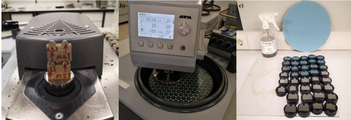
Figure 8. a) Bakelite process, b) Automatic sanding and polishing, c) Polished samples
