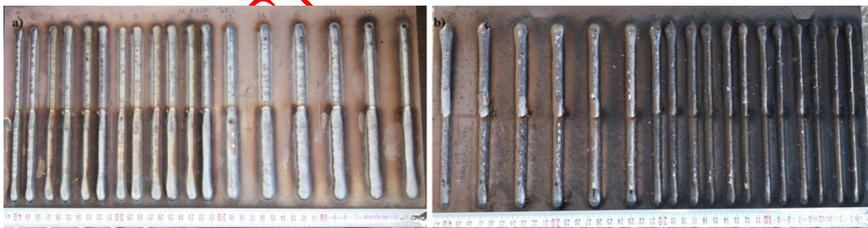
Figure 6. (a) Layers of solid wire, (b) Layers of metal-cored wire
