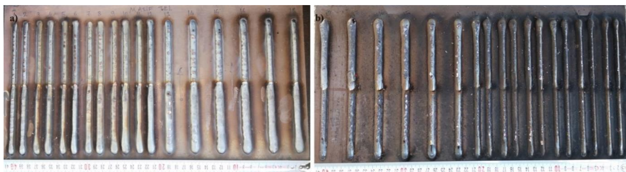
Figure 6. (a) Layers of solid wire, (b) Layers of metal-cored wire
