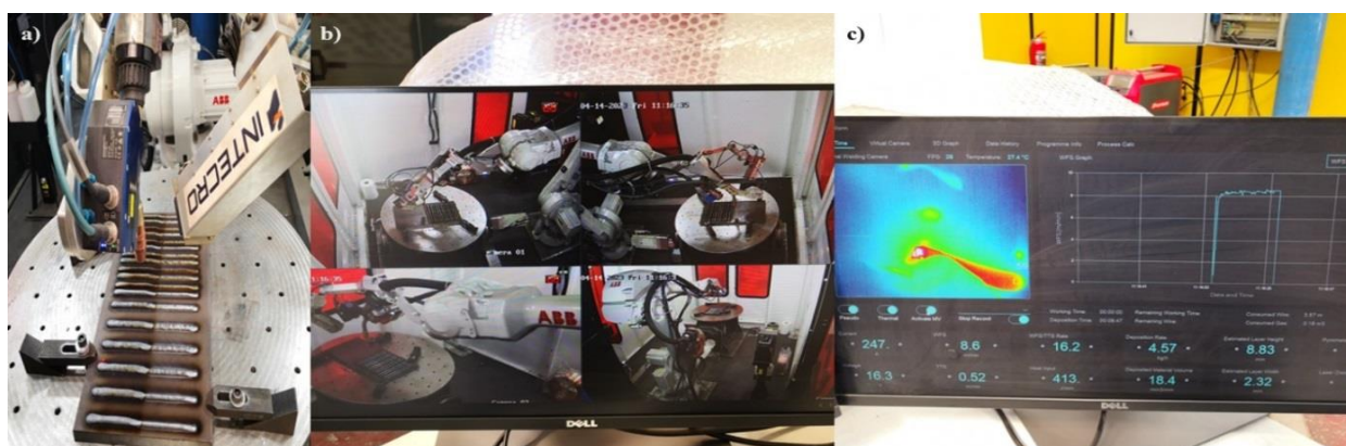
Figure 5. (a) Deposited beads, (b) Metalworm bench camera images (c) Metalworm digital control panel.
