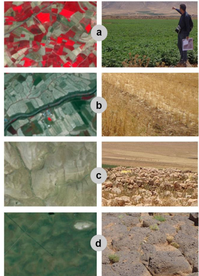
Figure 3. LU samples in the study area; a comparison between field and satellite image. a) irrigated crops (the light red color represents potatoes, while the dark red color corresponds to onions), b) rainfed croplands after harvest, c) basaltic terrains, d) limestone terrains.
