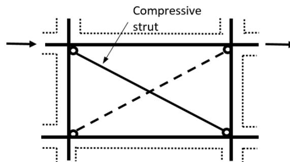
**Figure 1.** Model for infilled frames with a diagonal strut [10]
