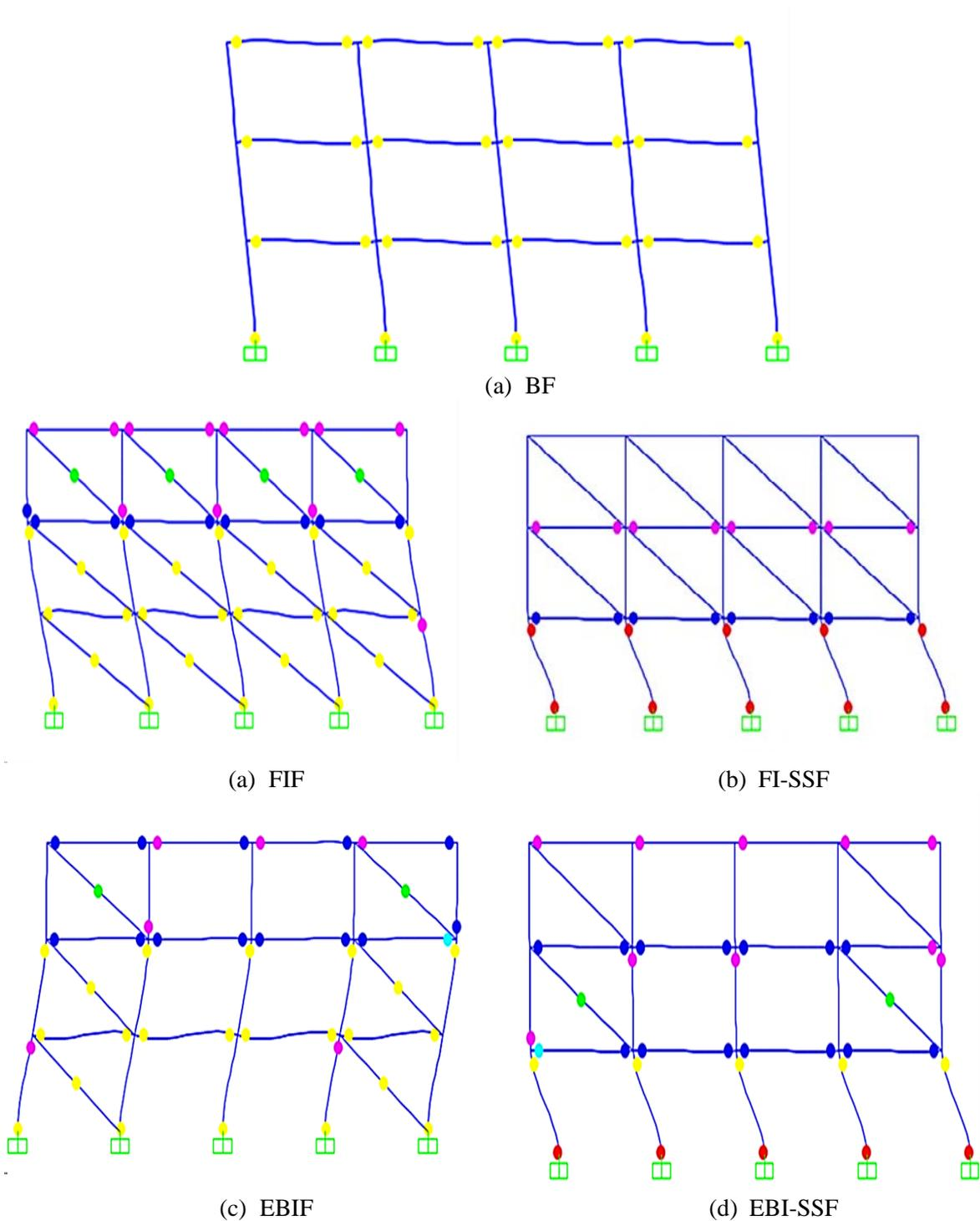
**Figure 9.** Plastic hinge distribution of 3 story-4 bay bare frame and infilled frames with  $t_w=25$  cm at failure
