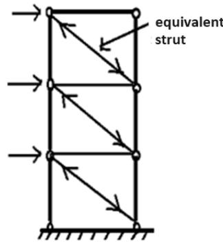
**Figure 2** Equivalent frame representation having infill panels [16]
