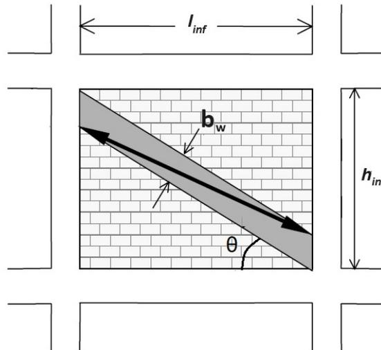
Figure 4. Strut placement in the frame model [18]
