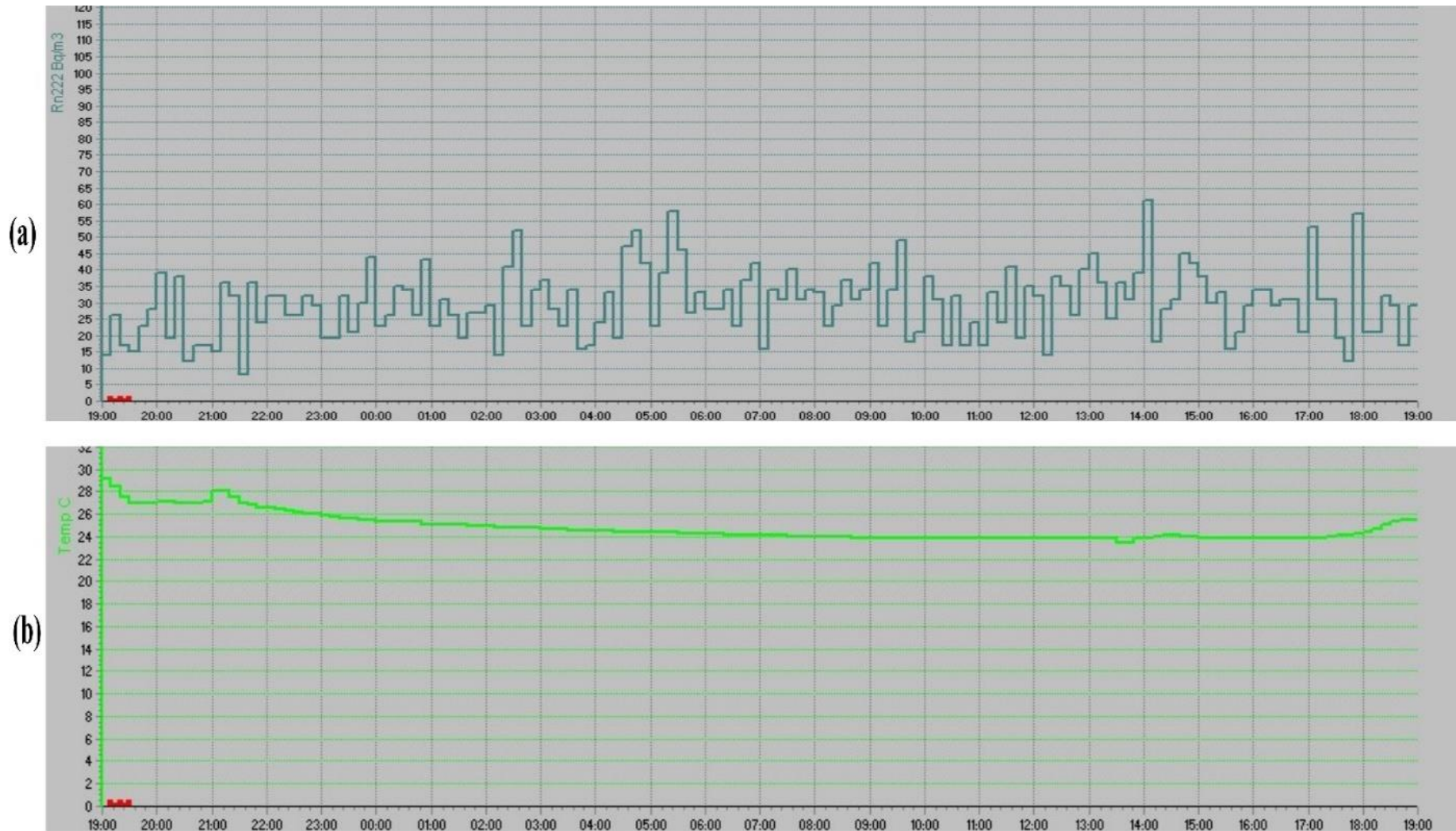
Figure 1. Sample graphs of measurements taken from the faculty building (a: ^{222}\text{Rn} activity concentration, b: temperature, c: pressure, d: relative humidity).
