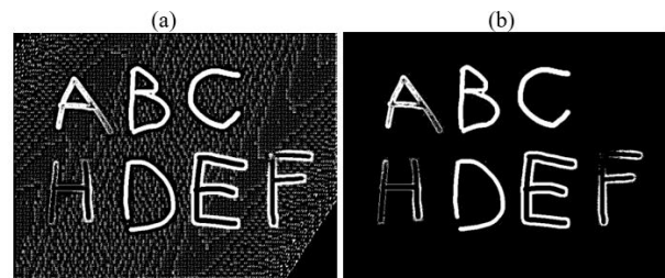
Figure 6. Difference of mean filter and normalization stages in the output matrix (a: mean filter matrix; b: normalization matrix)
