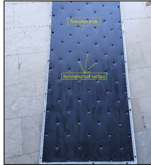
Fig. 7. Image of the the hemispherical absorber plate
