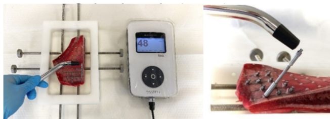
Figure 4. Measurement of the stability of mini-screws with the Ostell device.
