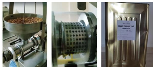
Figure 3. Process of extracting coriander seed oil using the cold pressing method.
