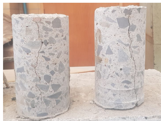
Fig. 6. Core samples reaching the full depth of the slab
