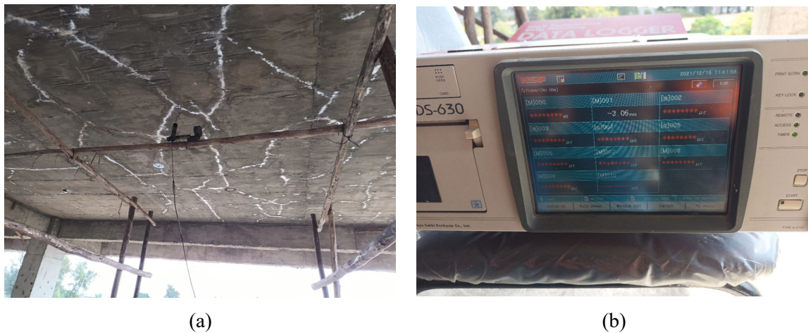
Fig. 3. Set-up for loading test (a) slab deflection measurement and (b) data logger
