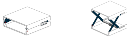
Figure 13. Closed and open state of the scissor system
