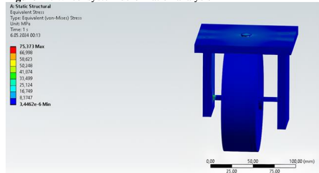
Figure 23. Wheel system stress analysis
