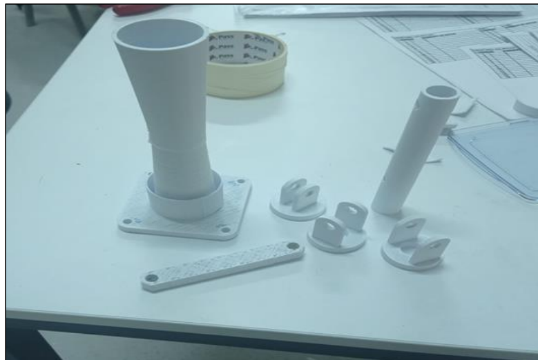
Figure 11. Parts produced by a 3D printer
