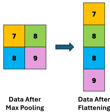
Figure 5. Example illustration of the size reduction transformation of the flatten layer
