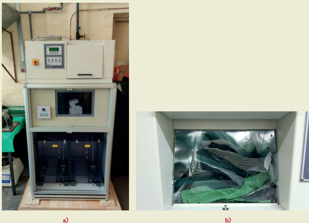
Figure 2. Solarbox xenon test chamber: a) the whole chamber, b) nets in the chamber
