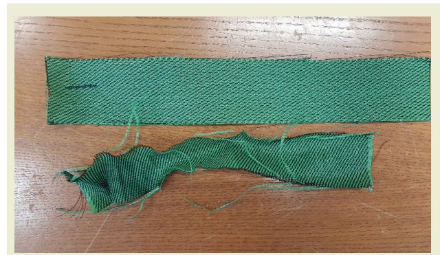
Figure 3. Curling of the nets after ageing
