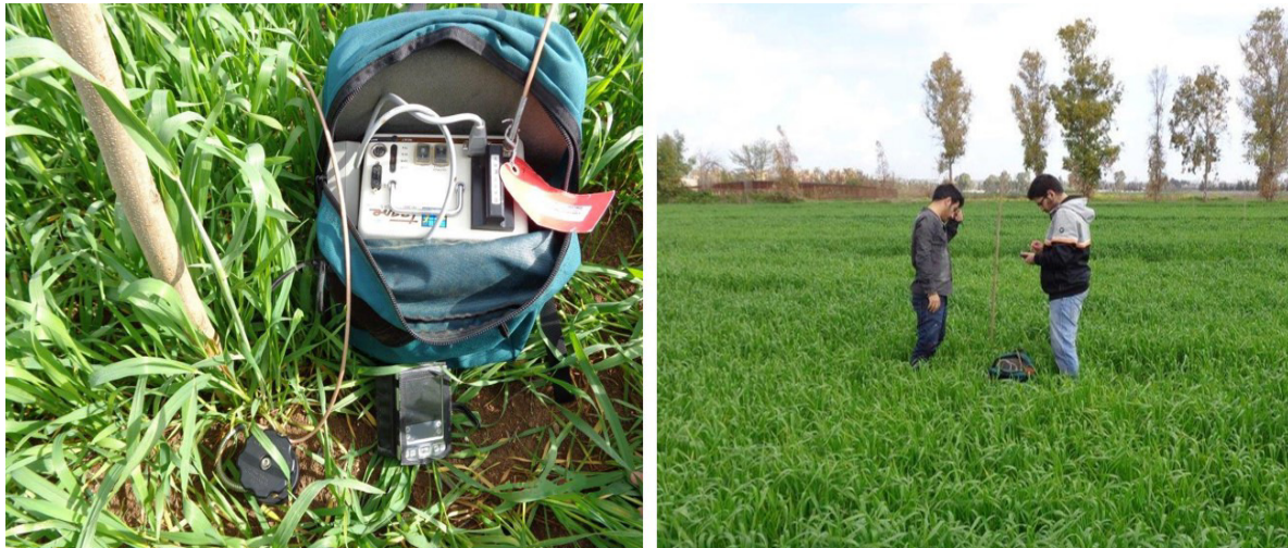
Figure 2. Measuring with time domain reflectometer (TDR) in experimental plots
