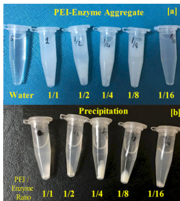
Figure 2 Images of PEI-enzyme aggregates with different concentrations of PEI from highest (1/1) to lowest ratio (1/16) and K. lactis lactase Lactozyme 2600L enzyme samples (1/300 dilution) before (a) and after (b) centrifugation (10,000 rpm for 2 minutes).
