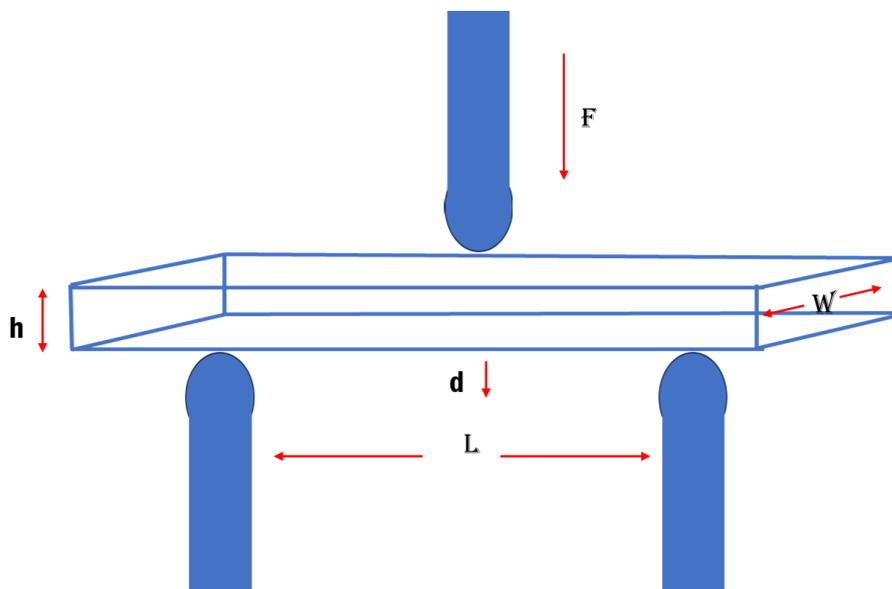
**Figure 1.** Diagram of the test design and definitions of the symbol of the formulas
