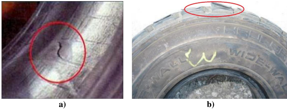
Figure 5. Defect types. a) crack defect b) Delamination defect [2]
