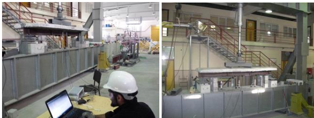
Figure 6. Steel-concrete composite beam test set-up
