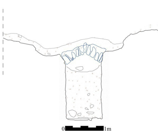
Figure 6: Cross-section drawing of the vault from the original phase of the aqueduct channel.
