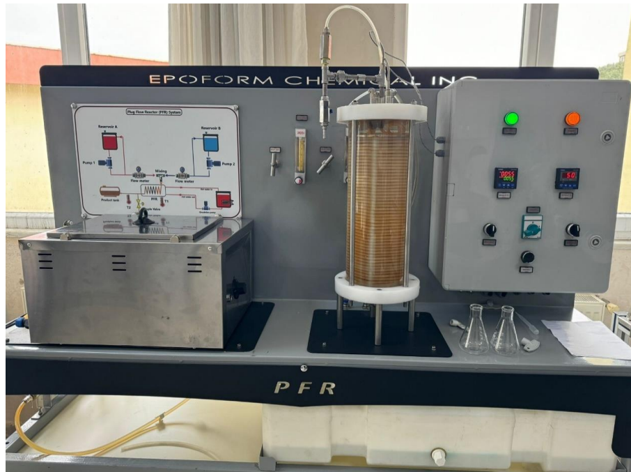
Figure 2. Experimental set-up of PFR
