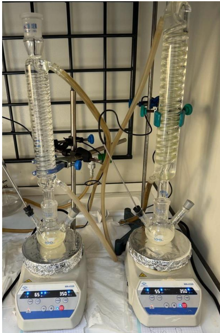
Figure 3. Experimental set-up of batch reactor
