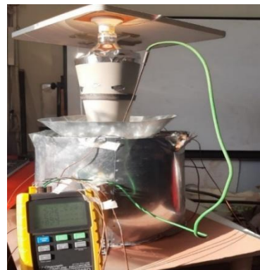
Figure 6. Schematic view of heat storage of Hitec salt by infrared lamp and its image in the experiment
