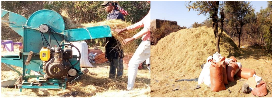
Figure 1. Field performance test of tef thresher during testing at Awash Melkassa wake Tiyo.
