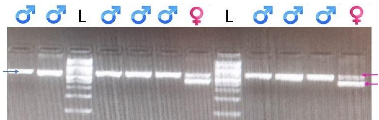
Figure 2. Gender identification was performed on 3% agarose gel electrophoresis. Out of ten parrots two were identified as female and eight as male from molted feather samples with using method 1. Female and male African grey parrots were observed with double (450bp and 600bp) and single (600bp) band patterns respectively (L: 100bp DNA ladder).
