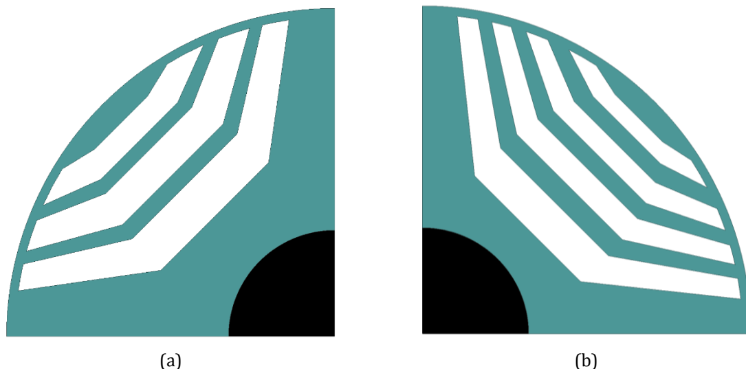
Figure 2. SynRM rotor structures (a) with 3 flux barriers and (b) with 4 flux barriers.
