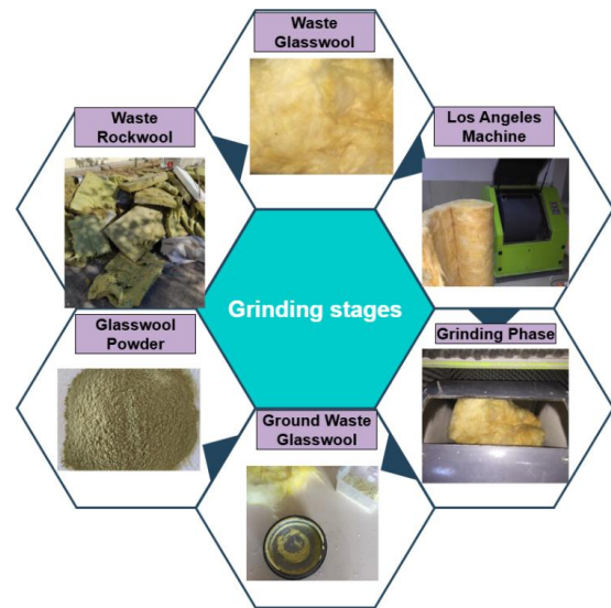
Figure 2. Grinding stages of mineral wool
