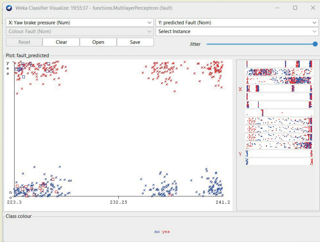
Figure 4. Relationship between Yaw Brake Pressure, and Failure Prediction
