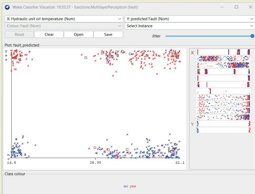
Figure 2. Relationship between Hydraulic Unit Oil Temperature, and Failure Prediction
