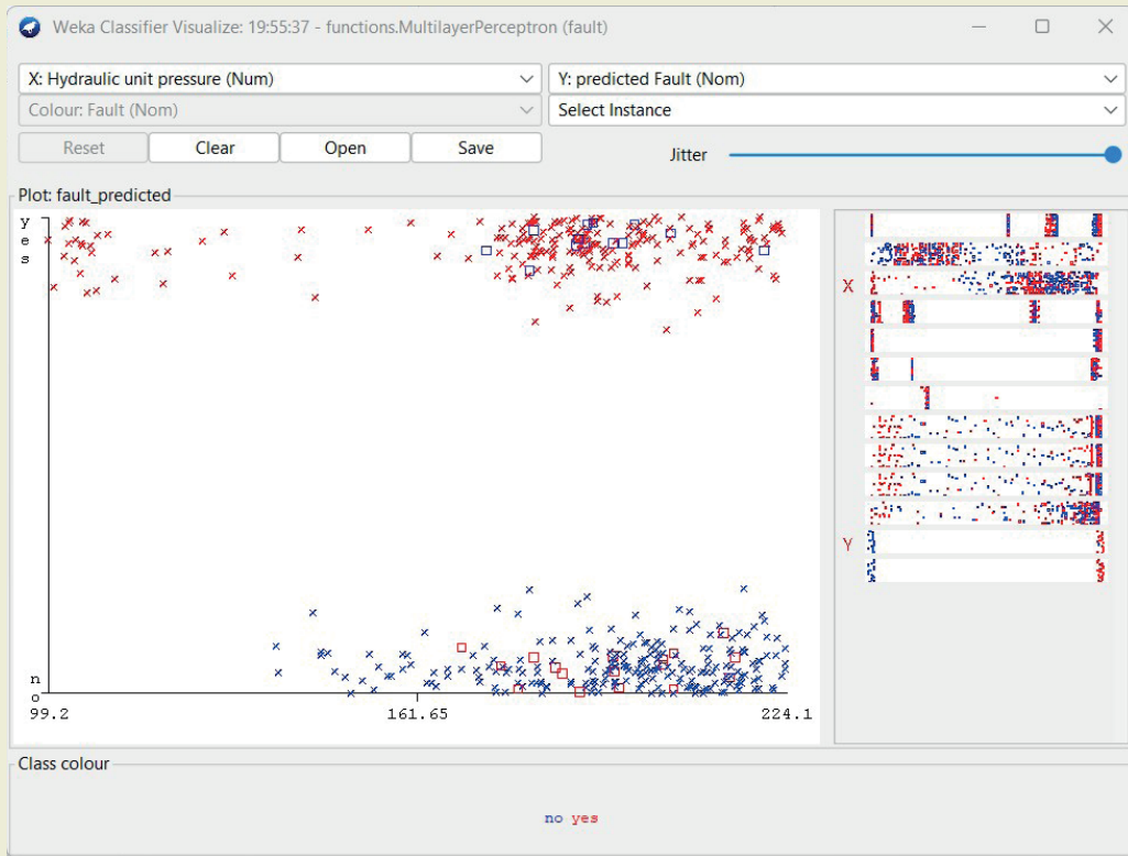
Figure 3. Relationship between Hydraulic Unit Pressure, and Failure Prediction
